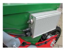
The speed of the high-torque motor is continuously adjustable via the controller.
