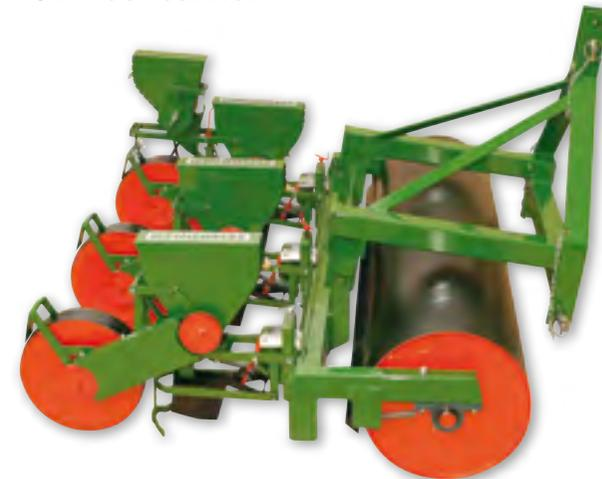
The tool carrier with the roller is particularly recommended for pre-rolling of loose soil to achieve an even seed depth.
