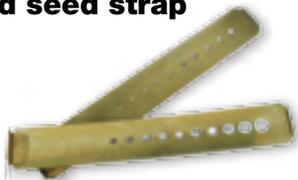
The HS and GSD seed drills use perforated seed straps to allow for precise and fast adjustment for seed size and/or seed rate. Two straps come with the HS hand pushed seeder and the GSD trailed seed drill.
